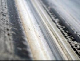
The belt was worn through the first two layers of fabric carcass leaving the third layer exposed and very vulnerable to further wear. The total width of the damage was 5.5 inches, length was 460 feet. Fortunately the damage was 6 inches from the edge of the belt and not in a high load bearing area. The repair needed to cover the exposed fabric in order to maintain belt integrity.
