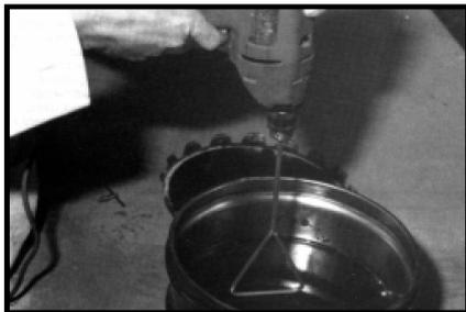
**5** Using stirring rod, mix resin and hardener thoroughly until a uniform color is obtained.
