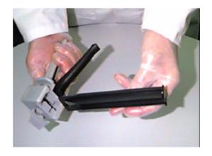
Assemble the gun as shown in the photographs. Unclip the cartridge retaining hinged bracket and insert the plunger into the gun handle, then insert the dual-barrelled cartridge into the retaining bracket, *ensuring that you hold the gun with the cartridge facing upwards to prevent bubbles returning to the resin*.
