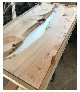
Nearly all river table designs feature some areas of resin that have no support and these areas require supporting whilst the resin is poured and throughout curing. It is very important that the barriers are totally sealed otherwise the resin will leak out.
