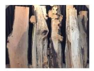
Ensure the wood is seasoned, dry and as flat as possible, a length of wood with a waney edge and interesting grain is ideal for this project. If you do not have the tools to cut the piece of wood the supplier will be able to do this for you. The piece of wood should be cut in half
