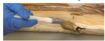
Leave this coat to dry but not completely cure. If the sealing coat is allowed to cure for more than 5 days then it must be lightly keyed with sand paper before pouring the rest of the resin or the two layers will not bond.
