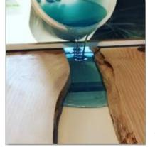
When pouring in multiple stages the best process is to allow the previous layer to cure to a firm but still tacky state, then pour the next layer on top of the partially cured layer.
