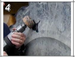
Grind the damaged area using a rubber grinding disk like the Rubber Exterminator. It is imperative you get a rough texture to allow for good adhesion.
