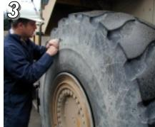
Skive out the rubber around the rip or tear. Be careful not to damage the steel radial of the tire with the blade
