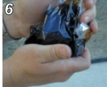
Open Eli-Flex FR909 kit, remove the spine and mix the two components together for 2-3 minutes or until warm. See "Six Easy Steps to Belt Repair" for more detailed instructions.
