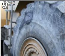
Allow 8 hours for Eli-Flex to cure. Buff as needed. See Tech Specifications for curing time at varying temperatures
