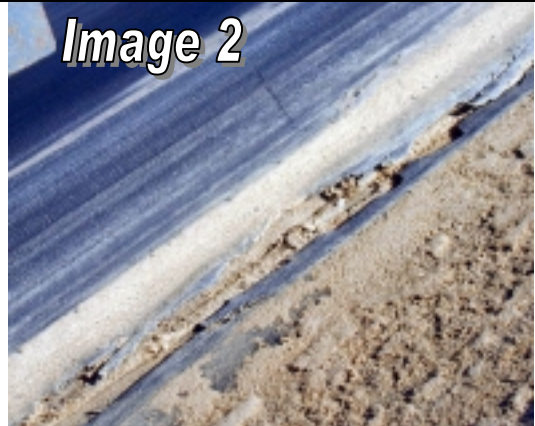
The damage was caused by age and running material with excessive weight over a belt with an idler configuration designed to handle a lighter load.
