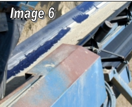
The depth of the repair was approximately 1/2 inch. The belt was operational within 3 hours of the repair
