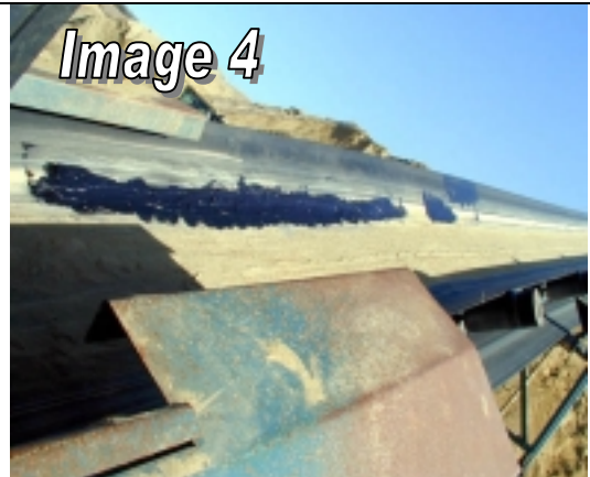
Total repair time was 30 minutes including cleaning and applying Eli-Flex.
